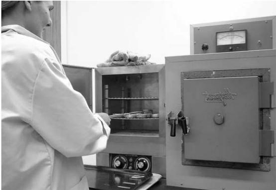
Lindsay, the Lab Technician, takes filters out of the drying oven. Next step is to weigh the filters, then to cook them at 500° C (932° F).
