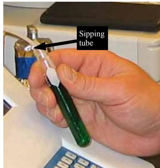
Close up of the ethanol-chlorophyll mixture being sipped into the fluorometer. The fluorometer quantifies the amount of light given off at a given wavelength.
