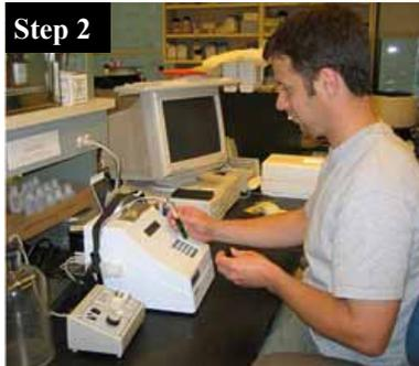
The ethanol-chlorophyll mixture is fed into a fluorometer and the readings are recorded for data entry.
