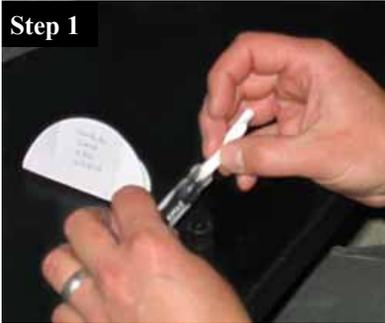
Chlorophyll filters are placed in a tube, ethanol is added, then the tubes are heated to extract the chlorophyll.
